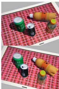
Flatbed 3-D Display (Above) Display viewed from left (Below) Display viewed from right The can with the orange and yellow cap, at the bottom right, is real; the other objects are generated by the display.
